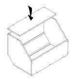
STEP 7 Upsdie down the cabinet, Turn the screw into the screw hole
